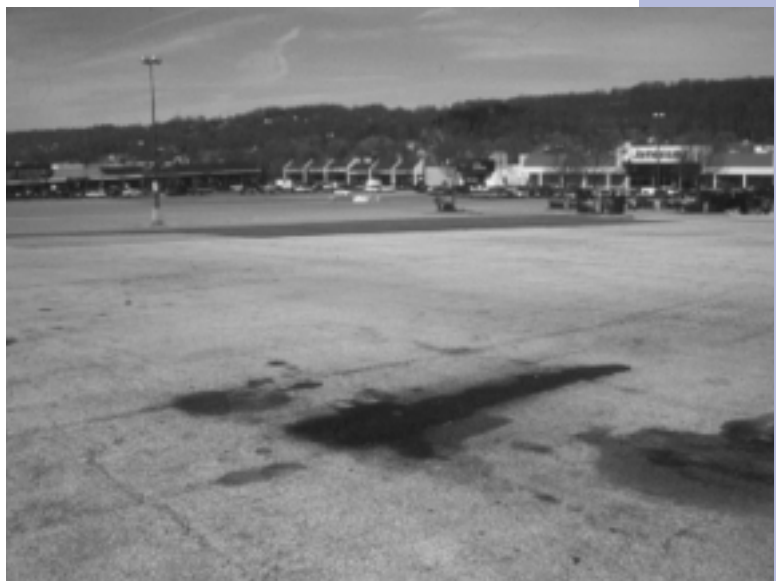
The increase of land area devoted to parking lots like this one in Chester County, PA, limit an area's ability to capture stormwater through ground absorption. Instead, stormwater flows from the man-made surfaces into local rivers and streams, where they impair water quality and make communities more susceptible to flooding. Photo courtesy of Chester County Water Resources Authority
